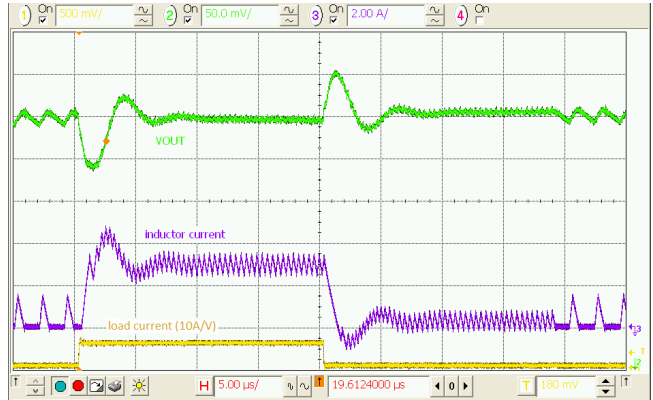
Figure 26. Load Transient, 3.6 V_{IN} , 1.2 V_{OUT} , 0.3–3 A, 100 ns Edge
