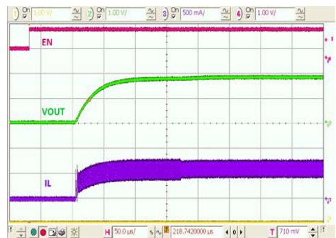
Figure 25. Startup, 3 \Omega Load
