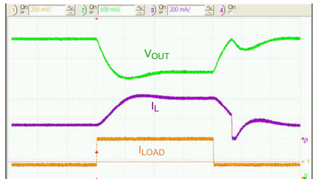
Figure 24. Load Transient 150 mA to 400 mA, V_{IN} = 3\text{ V} , t_{RISE} = t_{FALL} = 100\text{ ns} , 5\text{ }\mu\text{s/div} .
