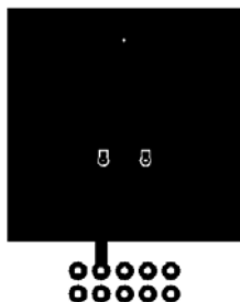
a) 40\text{ }^\circ\text{C/W} when mounted on a 1 in 2 pad of 2 oz copper
