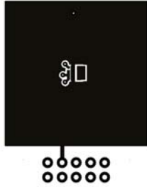
a. 65^\circ\text{C}/\text{W} when mounted on a 1 in 2 pad of 2 oz copper
