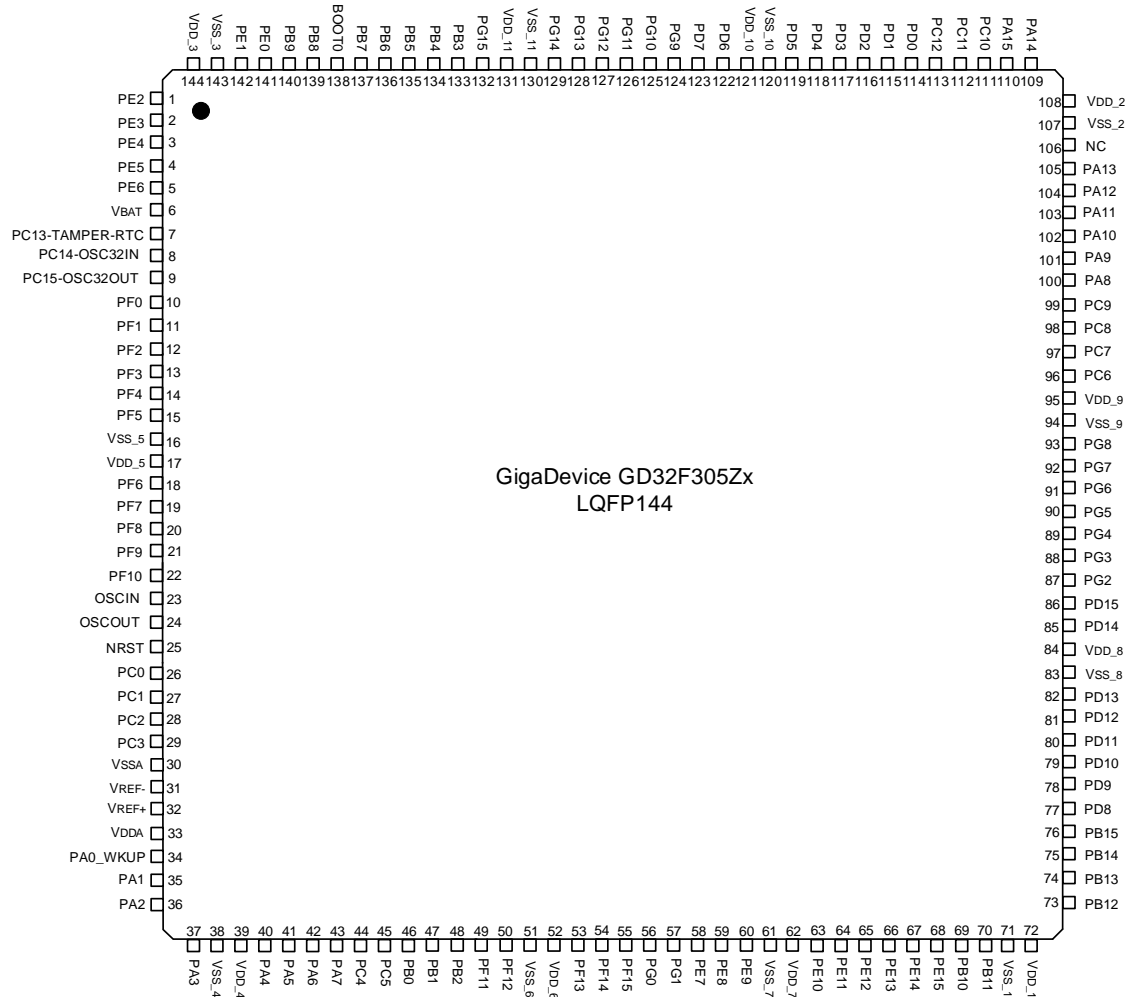
Figure 2-2. GD32F305Zx LQFP144 pinouts
