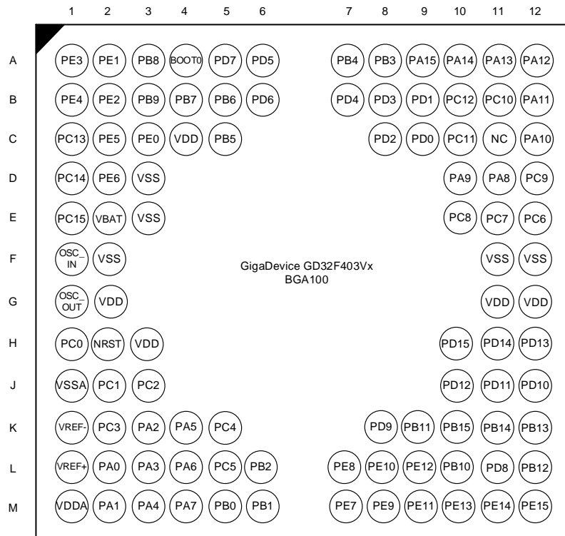
Figure 5. GD32F403Vx BGA100 pinouts
